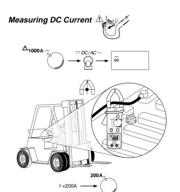
For greater accuracy on smaller currents, refer to the DC Zero procedure.
